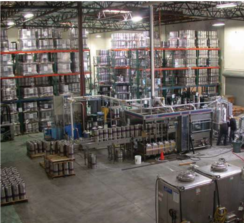
The fully automated KHS line sanitizes and fills the stainless kegs.
